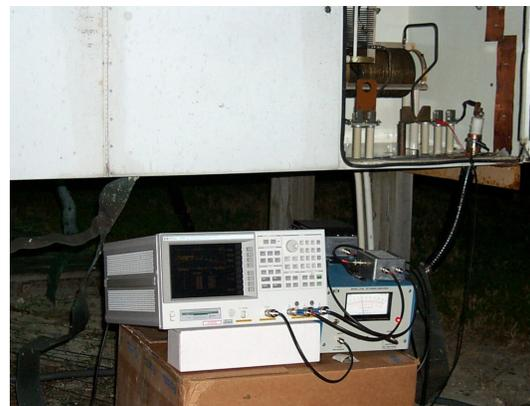
**Figure 3 – Impedance Measurements at ATU Input**
