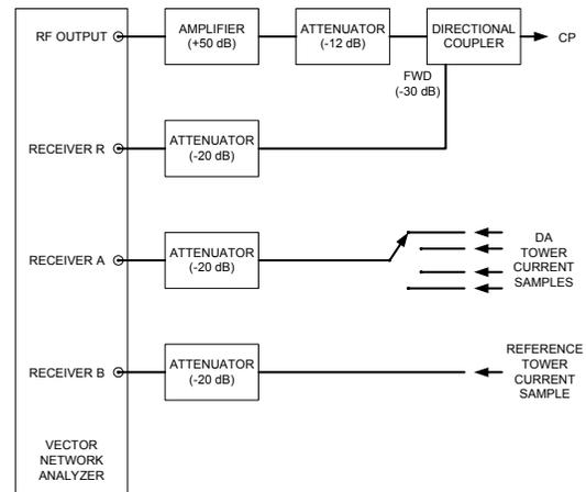
Figure 14 – DA Phase and Ratio Measurements
