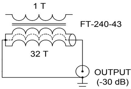
Figure 8 – Current Transformer
